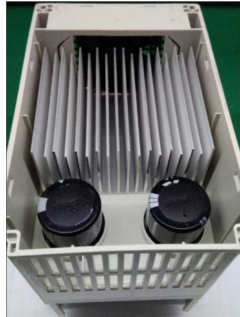
Two capacitors are installed bottom side for good cooling
