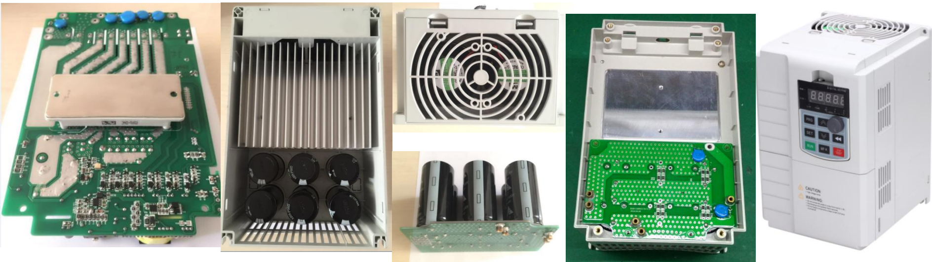
Infineon IGBT module, capacitors, big fans capacitors boards in bottom side SG3200, 11kw/15kw
